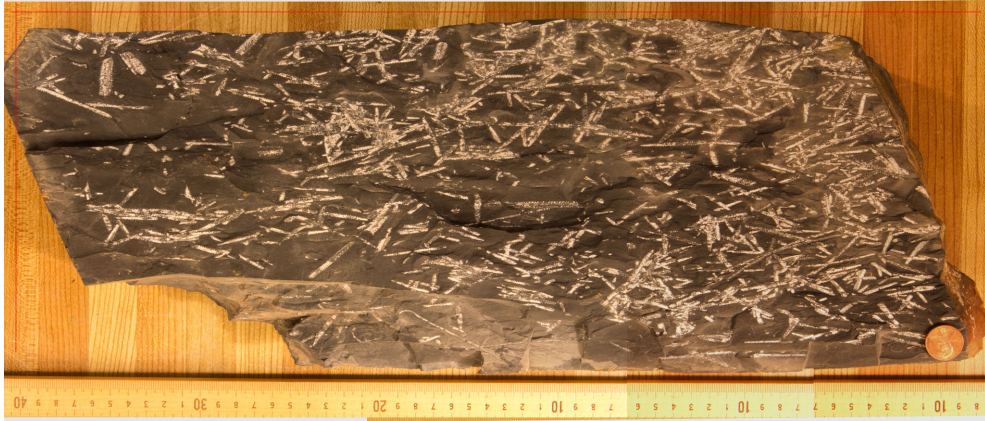
Figure 58. Sample of deformed graptoliferous slate used by Dirringer and Vollmer (2013) for comparison of the automated Wellman and mean polygon moment ellipse methods.
