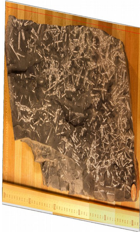
Figure 59. The graptoliferous slate sample of Figure 24 after retrodeforming to remove the strain calculated by the mean polygon moment ellipse method, R = 2.079 , \phi = 177.48^\circ
